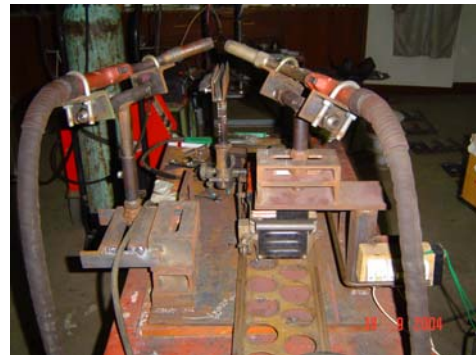
Figure 4. Welding jig and fixture
