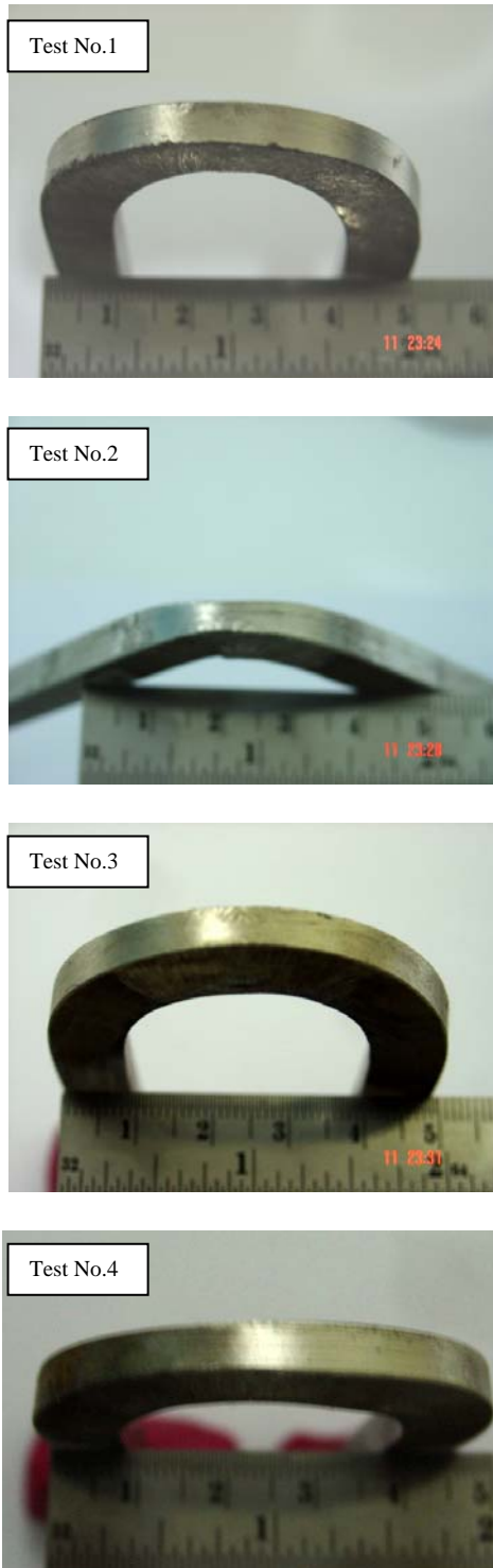
Figure 9. Side Bend Test, No Crack was found at all test pieces
