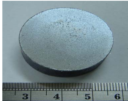
Figure 1. Forged billet of the Al-4wt.%Cu/15 vol.% Silica.
