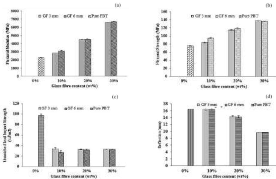
**Figure 3.** (a) flexural modulus (b) flexural strength (c) deflection and (d) impact strength of PBT and PBT/glass fiber composites.
