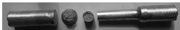
Figure 1. Picture of test specimen. In detail, the fracture surface can be viewed.
