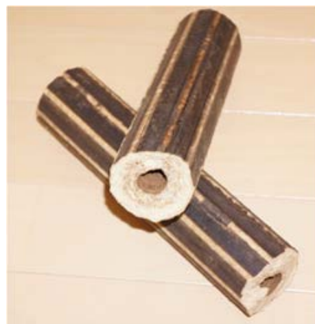
Figure 2. Compressed rice hull coke. (relative density: \sim 1.2 , water content: \sim 5.5\% )
