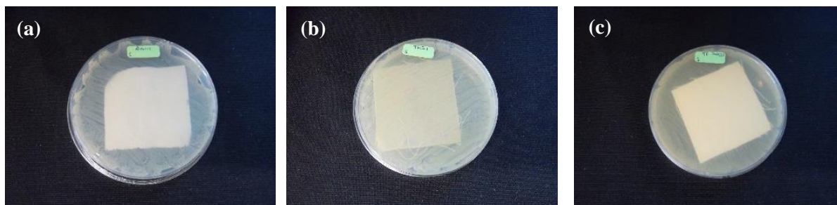
Figure 6. Images of samples tested according with the standard method JIS L 1902 (a) cotton fabric (b) 55:45 cotton-polyester blend fabric (c) 55:45 cotton-ZnO loaded polyester blend fabric.
