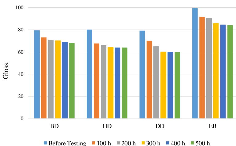
Figure 8. Gloss of cured screen printing ink films before and after weathering test.
