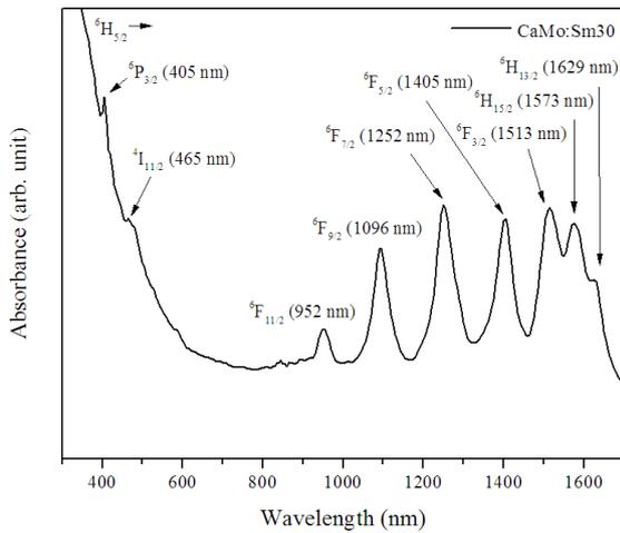
**Figure 3.** The absorption spectra of the CaMo:Sm30 phosphor in UV-Vis-NIR region.
