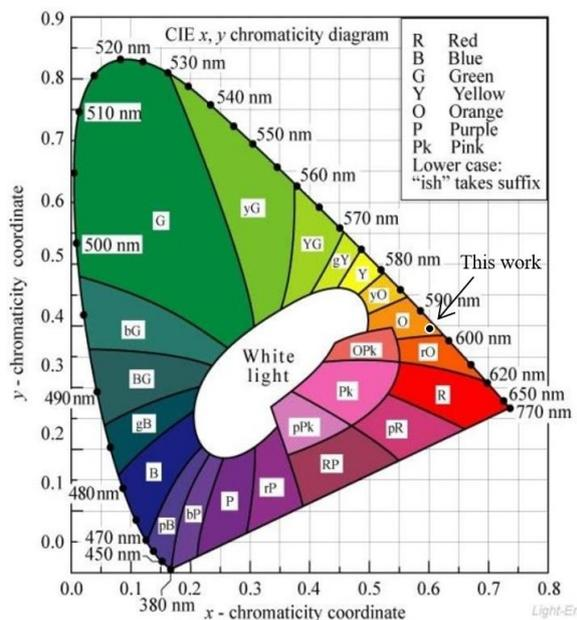
Figure 6. The CIE 1931 diagram of the  $\text{CaMoO}_4:\text{Sm}^{3+}$  phosphors.
