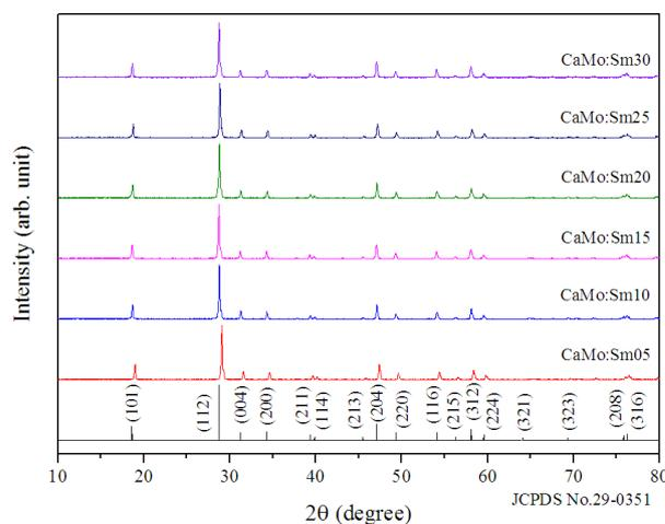
**Figure 2.** The XRD spectra of the  $\text{CaMoO}_4:\text{Sm}^{3+}$  phosphors.
