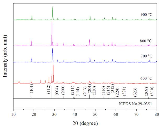
**Figure 1.** The XRD spectra of the  $\text{CaMoO}_4$  phosphors synthesized at different temperatures.
