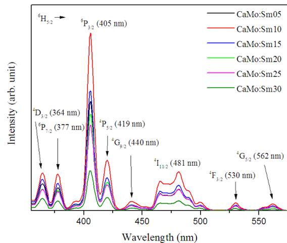
**Figure 4.** The excitation spectra of the CaMoO<sub>4</sub>:Sm<sup>3+</sup> phosphors observed with 600 nm.
