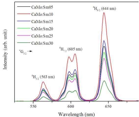
**Figure 5.** The emission spectra of the CaMoO<sub>4</sub>:Sm<sup>3+</sup> phosphors excited by 400 nm.
