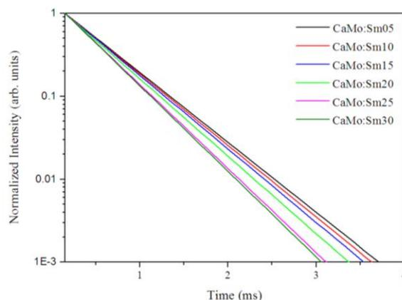
Figure 7. The decay curve of the  $\text{CaMoO}_4:\text{Sm}^{3+}$  phosphors for the  ${}^4\text{G}_{5/2} \rightarrow {}^6\text{H}_{9/2}$  transition.
