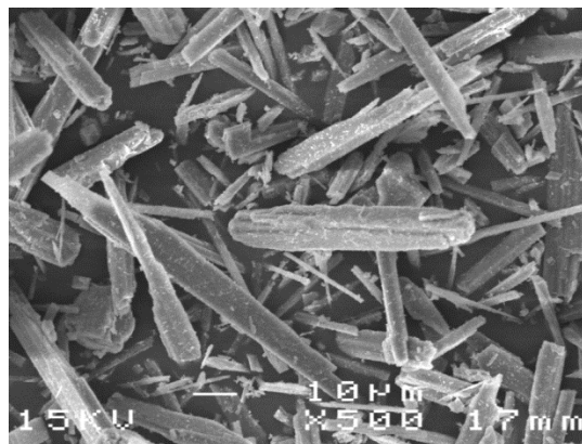
Figure 1. Representative SEM image of the ultrafine wollastonite ( \times 1,500 ).
