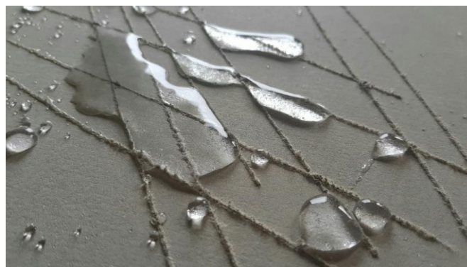
Figure 11. The actual fiber-cement board that used polyurethane-based corn starch–lithium perchlorate ( \text{LiClO}_4 ) as the additive.
