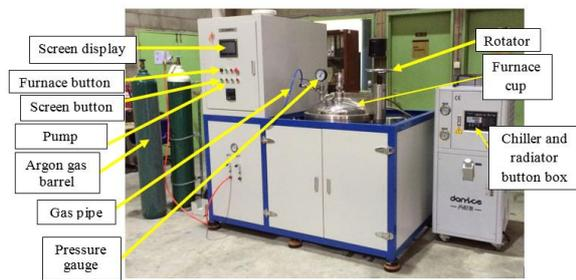
Figure 3. Microwave hybrid sintering furnace
