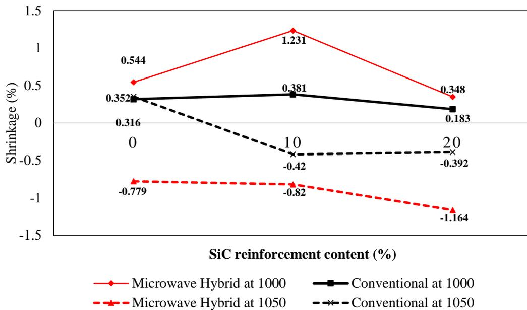
**Figure 4.** Shrinkage of pure Fe, Fe-10SiC and Fe-20SiC sintered by microwave hybrid and conventional at 1000°C and 1050°C.
