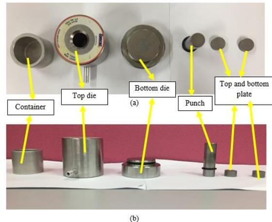
Figure 1. Cylindrical die parts (a) top view (b) side view.
