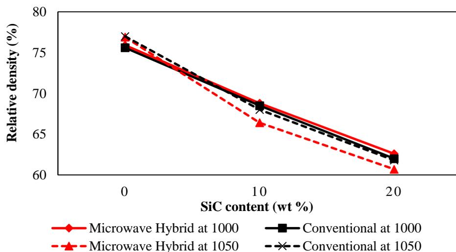
**Figure 5.** Relative density of pure Fe, Fe-10SiC and Fe-20SiC sintered by microwave hybrid and conventional method at 1000°C and 1050°C.
