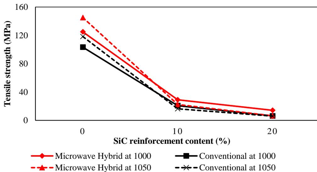
**Figure 7.** Tensile Strength of pure Fe, Fe-10SiC and Fe-20SiC sintered by microwave hybrid and conventional at 1000°C and 1050°C.
