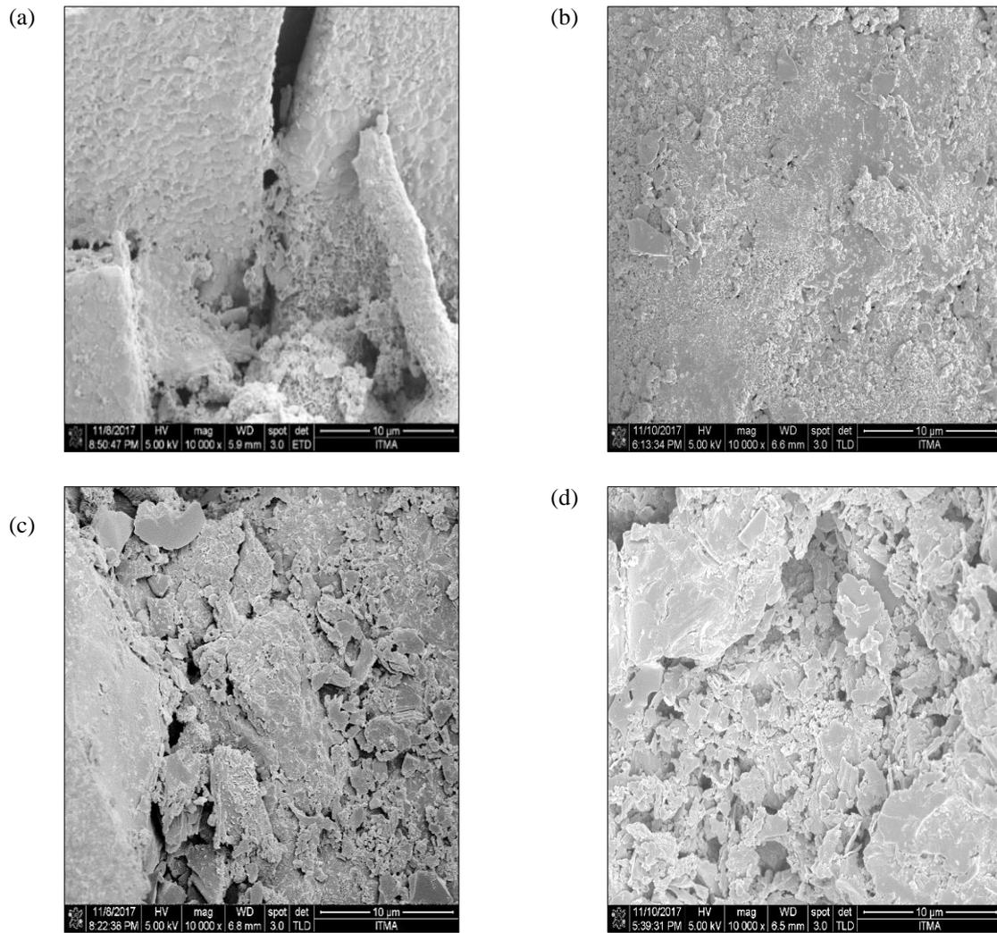
**Figure 6.** Fracture morphology experienced by the swelling sample (a) Fe-10SiC at 1050°C by microwave hybrid (b) Fe-20SiC at 1050°C by microwave hybrid (c) Fe-10SiC at 1050°C by conventional method (d) Fe-20SiC at 1050°C by conventional method.
