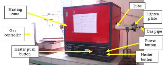
Figure 2. Vecstar tube furnace
