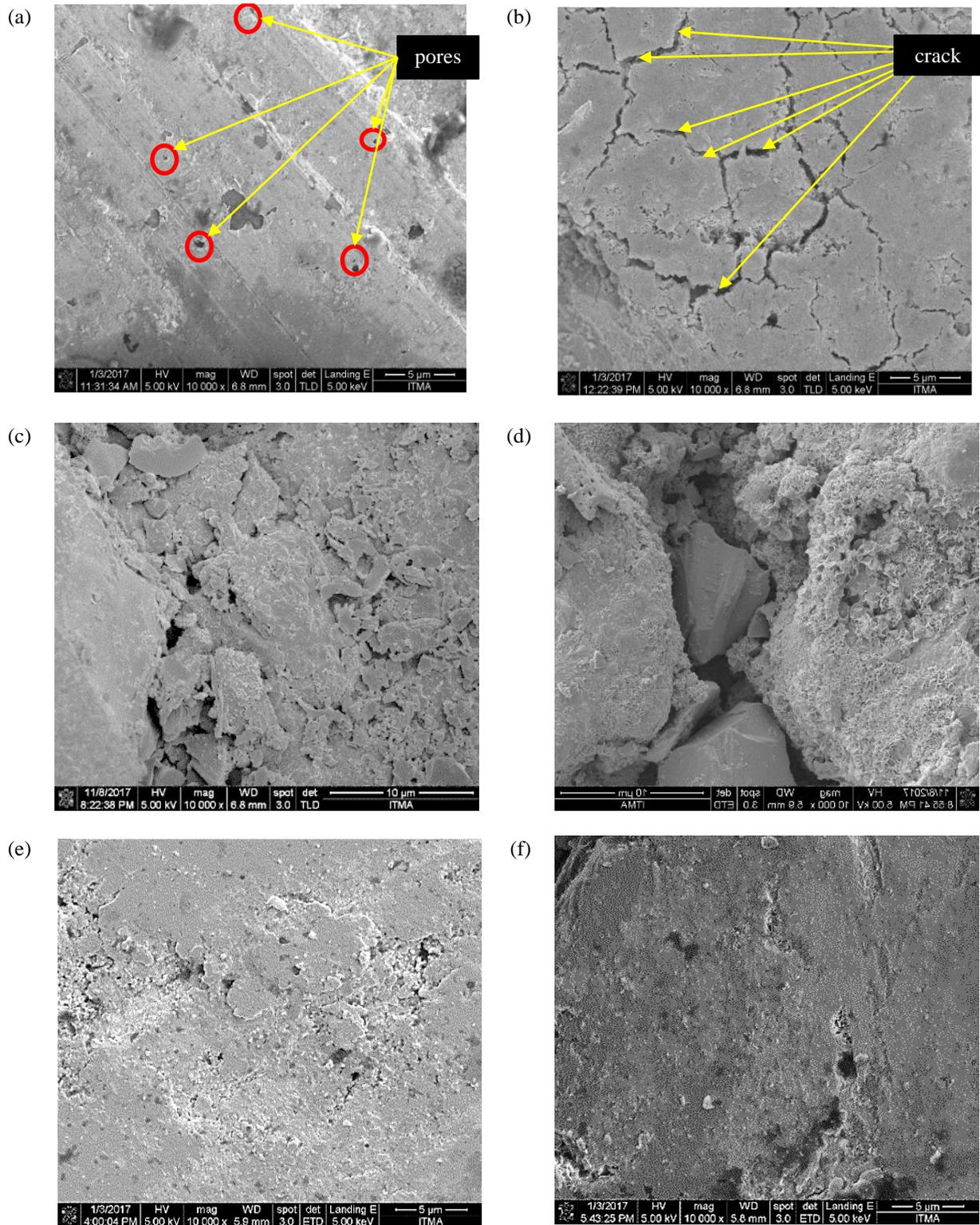
**Figure 8.** Microstructure of (a) Fe-10SiC at 1000°C by microwave hybrid (b) Fe-10SiC at 1000°C by conventional method (c) Fe-10SiC at 1050°C by microwave hybrid (d) Fe-10SiC at 1050°C by conventional method (e) Fe-20SiC at 1000°C by microwave hybrid (f) Fe-20SiC at 1000°C by conventional method.
