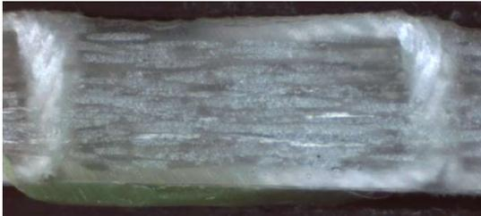
**Figure 1.** Microscopic image of tufted composites.
