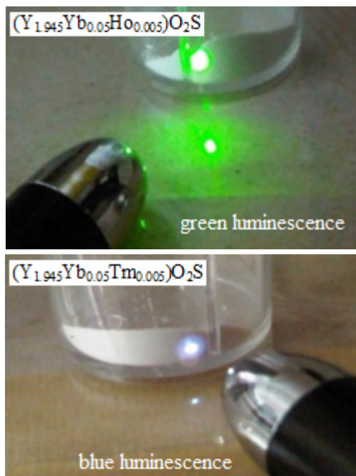
Figure 4. The upconversion luminescence of co-doped Y_2O_2S samples excited by 980 nm laser pen.
