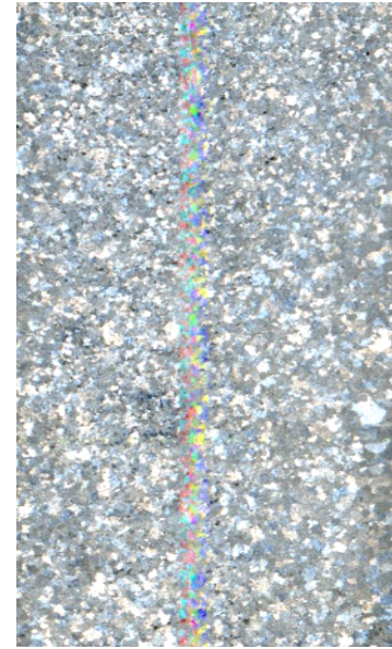
Figure 4. Macrostructure of Al-20Sn
