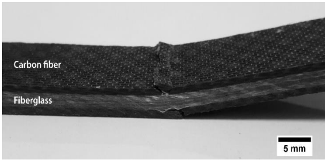
Figure 8. An example of a broken SWFG specimen after flexural properties testing. The upper carbon fiber skin buckles up against the folding direction due to compression.
